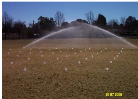
A 'catch can' test measuring sprinkler efficiency.
