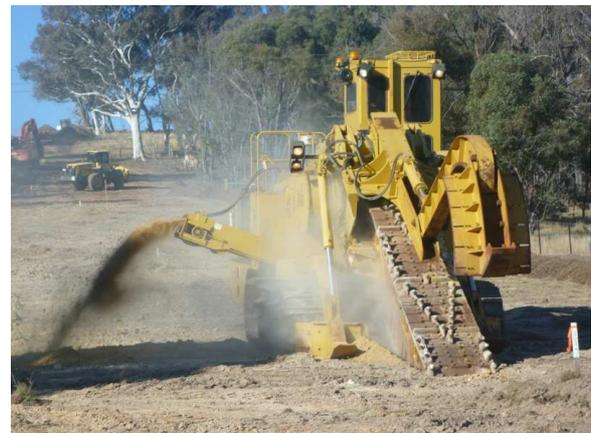
**Figure 2 Trenching machine excavating adjacent to the Monaro Highway**
